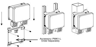
Warning: The mounting column must be anchored at both ends: floor and ceiling.
