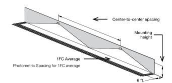
Industrial environment: Wall mounted equipment, reflectances: 10/10/10; 6-ft wide illumination path. Illumination as per NFPA101; Average: 1fc; Min: 0.1fc; Max/min< 40:1
