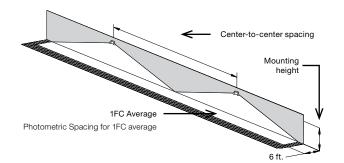
Industrial environment: Wall mounted equipment, reflectances: 10/10/10; 6-ft wide illumination path. Illumination as per NFPA101; Average: 1fc; Min: 0.1fc; Max/min< 40:1
